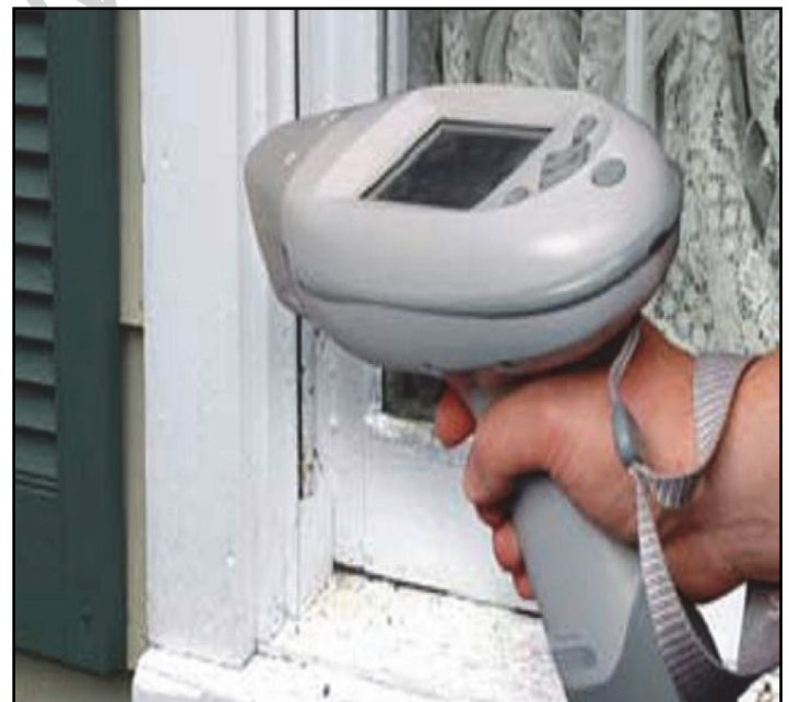
Photo 3: On-site XRF analysis can be helpful for locating corrosive drywall panels, but several factors must be considered in data interpretation.
