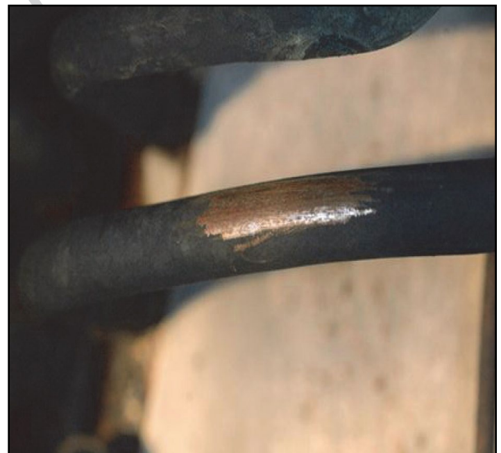
Photo 2: Blackening of copper surfaces indicates sulfur corrosion.
