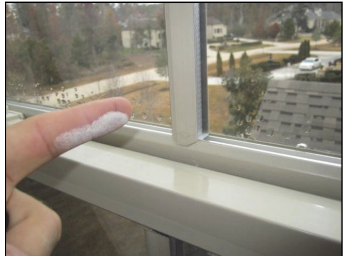
Photo 7: Inspector identifies visible dust after attempted cleanup. The presence of dust indicates that additional work is required.
